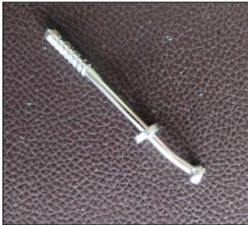
Figure 8: Picture of the bent screw.
